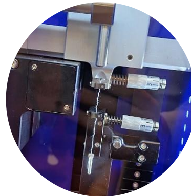
Measuring the elasticity in the yarn
